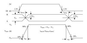
Figure 7. Driver Propagation Delays
