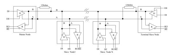
Figure 1. Typical Half-Duplex RS-485 Network
