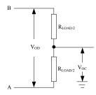
Figure 2. Driver DC Test Load
