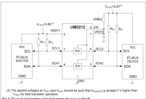
Fig 2. Typical application circuit (switch always enabled)
