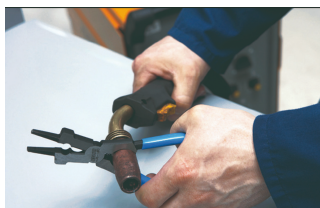
Nozzle removal and installation
