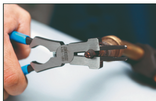
Tip removal and installation
