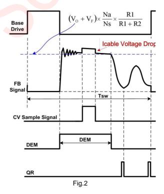
During the CV sampling process, an internal variable current source is flowing to FB pin for Cable Drop Compensation (CDC). Thus, there is a step at FB pin in the transformer demagnetization process, as shown in Fig.2.
