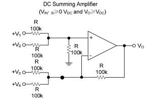
Where:  $V_0=V_1+V_2-V_3-V_4$ ,  $(V_1+V_2) \ge (V_3+V_4)$  to keep  $V_0>0 V_{DC}$
