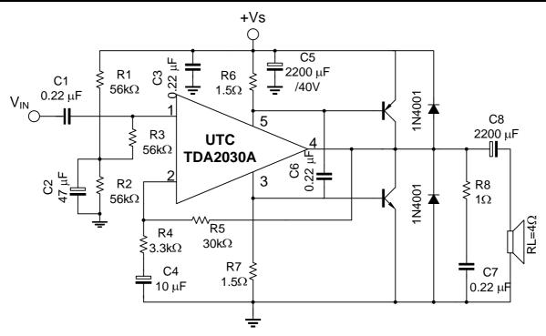
Fig. 1 Single supply high power amplifier
