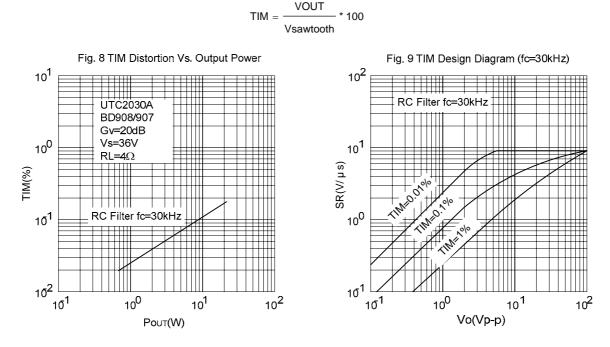
In Fig.8 The experimental results are shown for the 30W amplifier using the **UTC TDA2030A** as a driver and a low-cost complementary pair. A simple RC filter on the input of the amplifier to limit the maximum signal slope(SS) is an effective way to reduce TIM.
