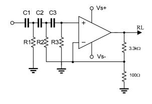
The components values calculated for fc=900Hz using a Bessel 3rd Sallen and Key structure are:
