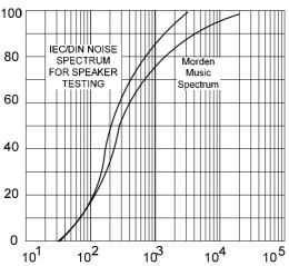
Fig. 2 Power Distribution vs. Frequency
