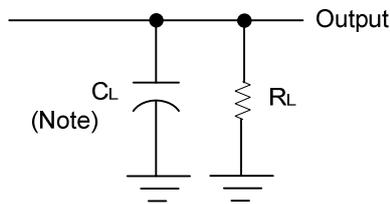
Note:  $C_L$  includes probe and jig capacitance.
