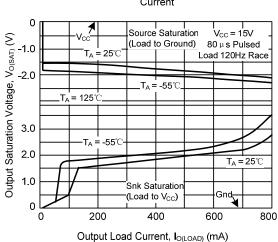
Output Saturation Voltage vs. Output Load Current
