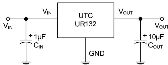
The part may oscillate without the capacitor, a 10µF (or larger) capacitor is recommended between  $V_{OUT}$  and GND for stability. Any type of capacitor can be used, but not Aluminum electrolytic when operating below -20°C. The capacitance may be increased without limit. Besides, another 1µF capacitor (or larger) should be placed between  $V_{IN}$  to GND.
