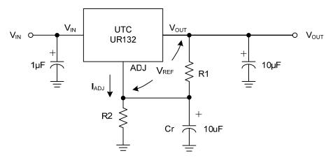
Cr:10 $\mu$ F to improve ripple rejection  $V_{OUT}=V_{REF}(1+R2/R1)+I_{ADJ}xR2$
