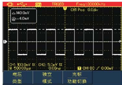
图6-29 电压光标测量菜单
