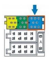
Illustrative view of the back of the MFD radio to which you must connect the AUDIO adapter.
