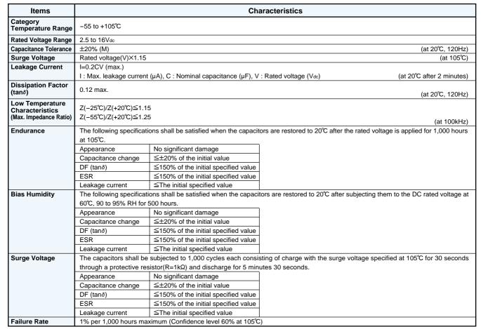
\*Note: If any doubt arises, measure the leakage current after following voltage treatment.
