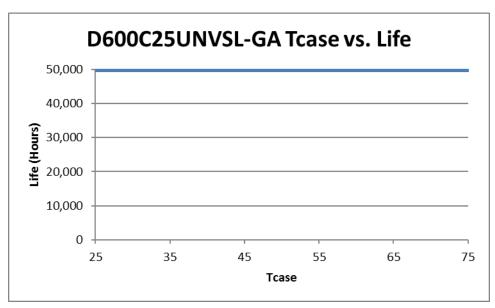
The Data curve provided predicts the LED Driver life based on the case temperature measured at the Tc location identified on the label or specification sheet. The Telecordia SR-332 standard is used to generate the prediction curves.
