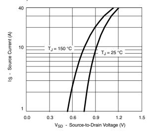
Source-Drain Diode Forward Voltage
