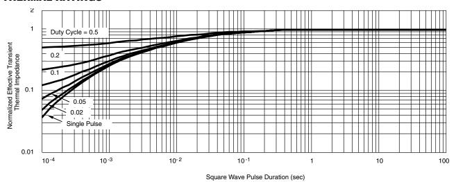
Normalized Thermal Transient Impedance, Junction-to-Case
