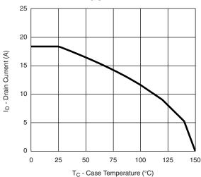
Maximum Drain Current vs. Case Temperature
