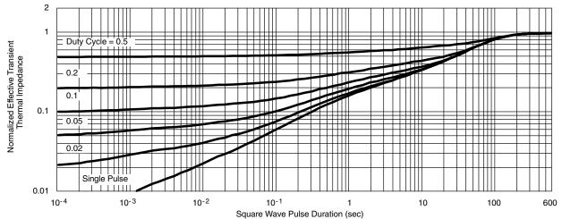
Normalized Thermal Transient Impedance, Junction-to-Ambient
