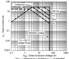
\* V<sub>GS</sub> > minimum V<sub>GS</sub> at which r<sub>DS(on)</sub> is specified **Safe Operating Area**
