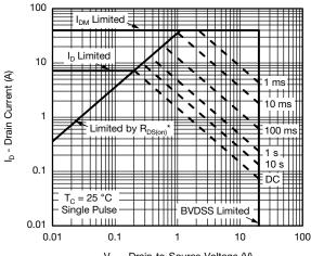
$$\begin{split} &V_{DS}\text{ - Drain-to-Source Voltage (V)}\\ ^*V_{GS}> &\min \text{mum }V_{GS}\text{ at which }R_{DS(on)}\text{ is specified}\\ &\textbf{Safe Operating Area} \end{split}$$
