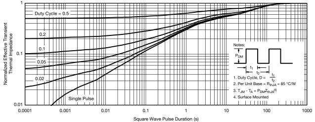
Normalized Thermal Transient Impedance, Junction-to-Ambient
