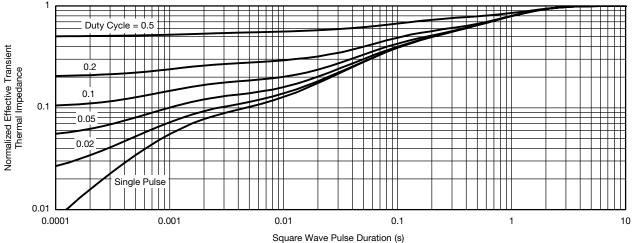
Normalized Thermal Transient Impedance, Junction-to-Foot
