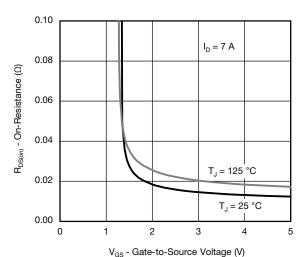
On-Resistance vs. Gate-to-Source Voltage
