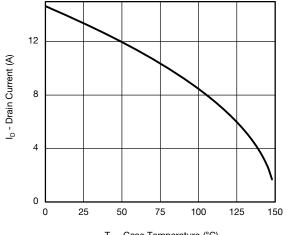
T<sub>C</sub> - Case Temperature (°C) **Current Derating\***
