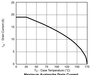
Maximum Avalanche Drain Current vs. Case Temperature
