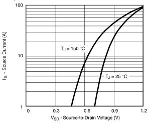
Source-Drain Diode Forward Voltage
