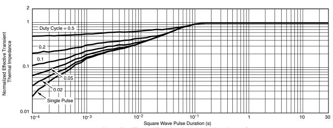
Normalized Thermal Transient Impedance, Junction-to-Case
