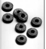
Multi-functional solder washer kits, with three sizes of washers. Different sizes provided to fit over sockets and tails of most Vector socket pins and wiring terminals. Ideal tools for committing pins to voltage and ground planes in Vectorbord patterns, such as Voltage/Ground Plane and Vectorbord plus ™, that have clearance area isolating holes from planes.
