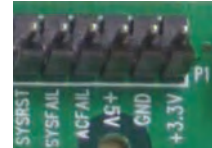
6-Pin Utility Connector On rear of Backplanes
