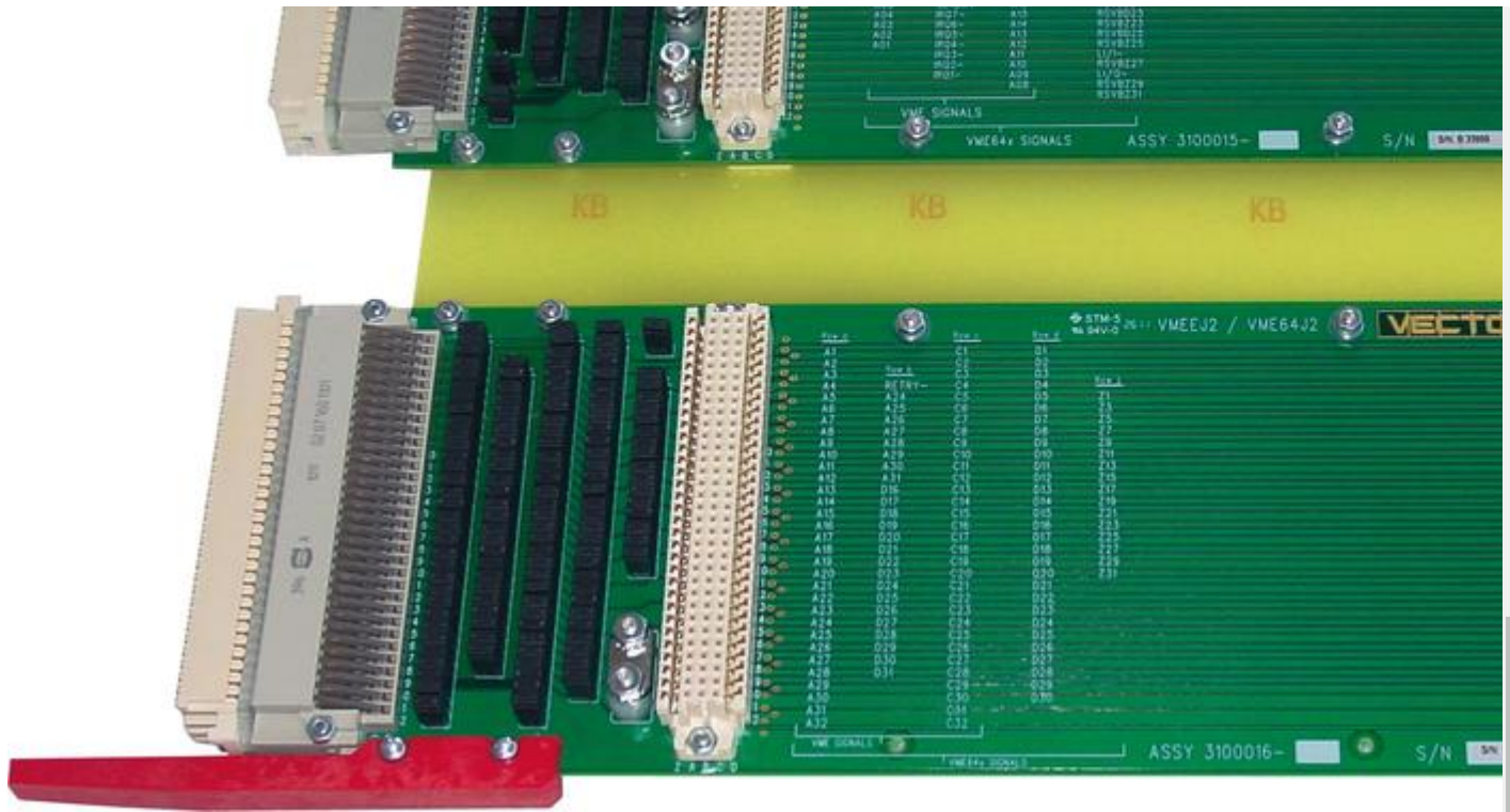
6U Overall, VME64x J1/J2 (without J0) with 5-row, 160 positions DIN 4161 connectors
