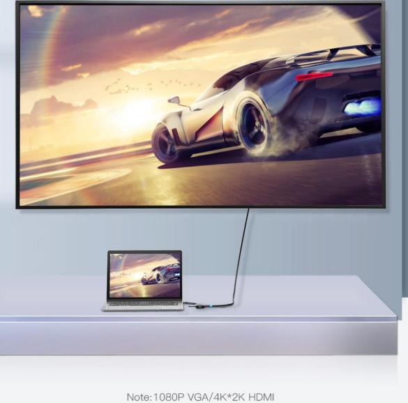
When HDMI and VGA output simultaneously, the resolution is 1080P@60Hz
