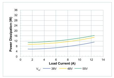
**Figure 5** — Power dissipation at  $T_{CASE} = -40$ °C
