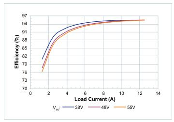
**Figure 4** — Efficiency at  $T_{CASE} = -40$ °C
