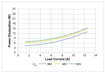
**Figure 9** — Power dissipation at T<sub>CASE</sub> = 100°C
