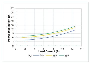
**Figure 7** — Power dissipation at  $T_{CASE} = 25^{\circ}C$
