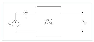
**Figure 17** — K = 1/2 Sine Amplitude Converter with series input resistor
