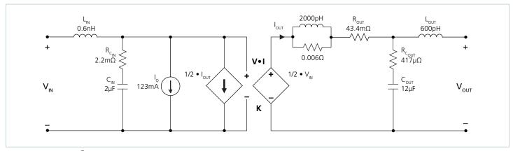
Figure 16 — VI Chip® module AC model
