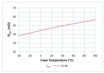
**Figure 10** — R<sub>OUT</sub> vs. temperature; nominal input
