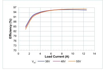
**Figure 6** — Efficiency at  $T_{CASE} = 25$ °C
