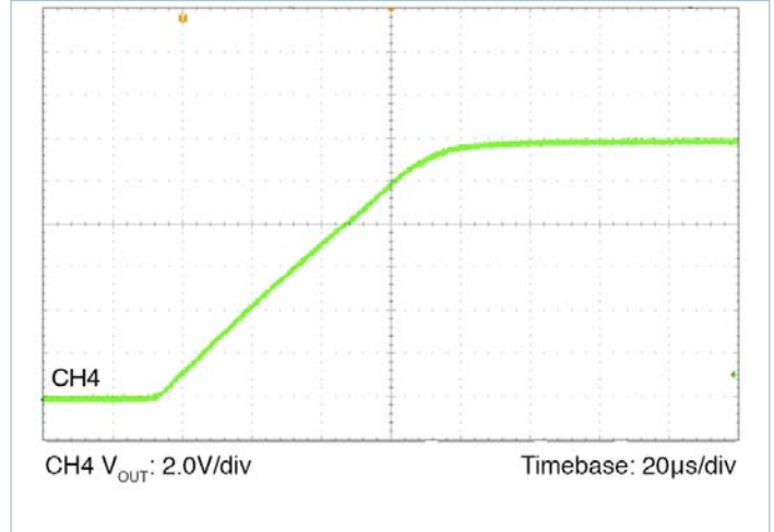
Figure 8 — Output voltage rise time at nominal line, 10% load, 0 capacitance
