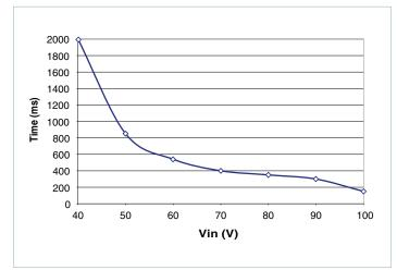
Figure 3 — Shut-down time of M-FIAM9 vs. overvoltage
