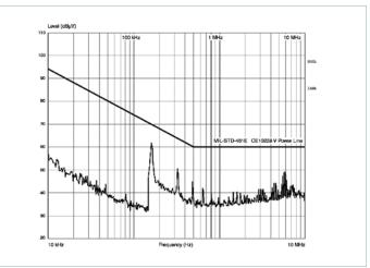
Figure 2 — Conducted noise: M-FIAM9 and model V28A12M200B DC-DC converter operating at 28V<sub>DC</sub>, 200W
