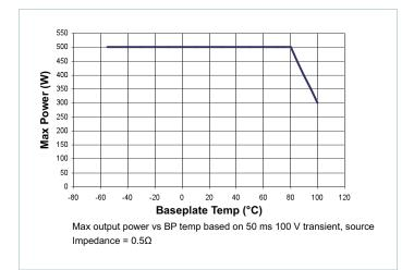
Figure 5 — Temperature de-rating
