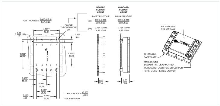
Figure 9 — PCB mounting specifications
