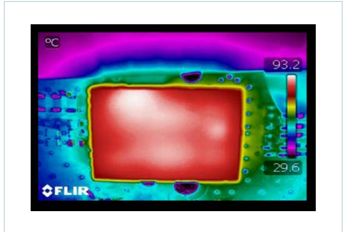
Figure 10 — Thermal image ( V_{IN} = 24V , I_{OUT} = 10A , CR, OLFM evaluation PCB)
