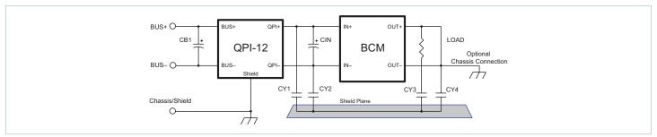
Typical QPI-12 application schematic with Vicor BCM module [a]
