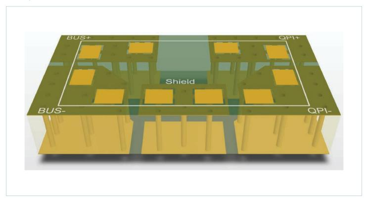
**Figure 22** — 3D view of paralleling planes underneath the QPI-12
