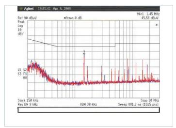
Figure 6 — VTM V048F480T006-CB with 153W load
