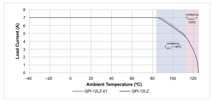
Figure 11 — Current de-rating over ambient temperature range
