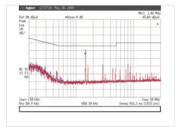
Figure 5 — VTM V048F240T012-CB with 172W output load
