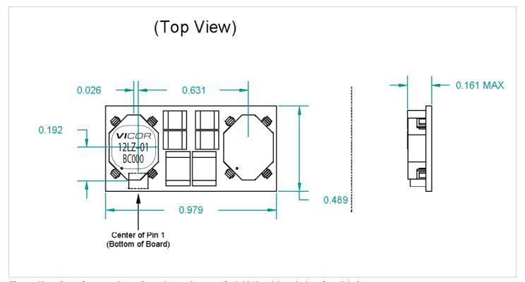
**Figure 19** — Open-frame package dimensions, tolerance of ±0.004in; pick-and-place from label center
