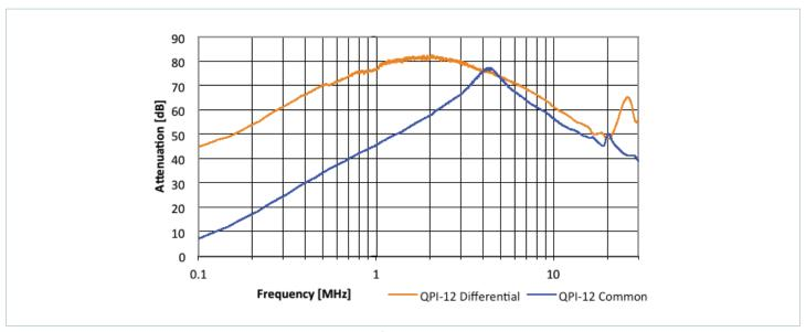
**Figure 15** — Attenuation curves into a  $50\Omega$  line impedance, bias from a 48V bus
