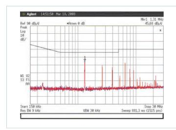
Figure 7 — BCM B048F030T21-EB with 160W load
