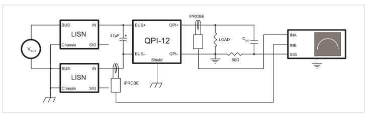
Figure 16 — Test set up to measure differential-mode EMI currents in Figure 15
