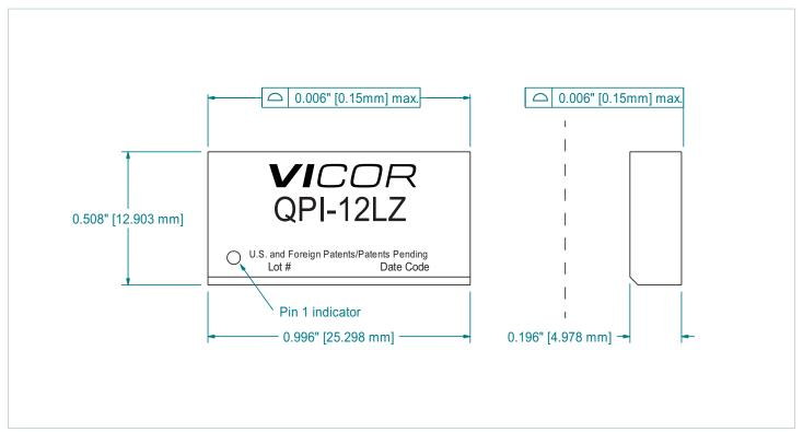
Figure 18 — Lidded package dimensions, tolerance of ±0.004in
