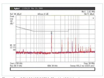
Figure 8 — BCM B048F120T30-EB with 180W load
