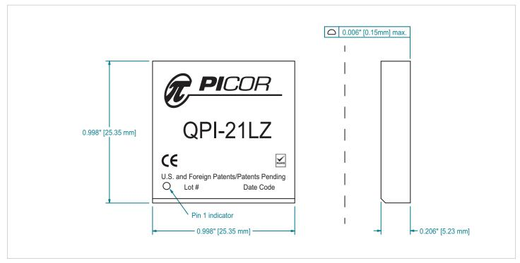
Figure 20 — Lidded Package Dimensions, tolerance of ±0.004"
