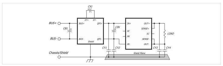
Figure 2 — Typical QPI-21 circuit with a Vicor brick converter. Optional X (CX1) filter capacitor shown. [b]
