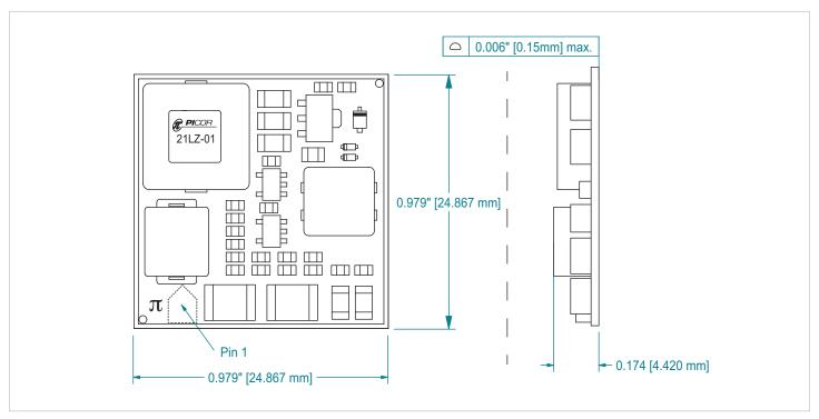
Figure 21 — Open-frame Package dimensions, tolerance of ±0.004". Pick and Place from label center.
