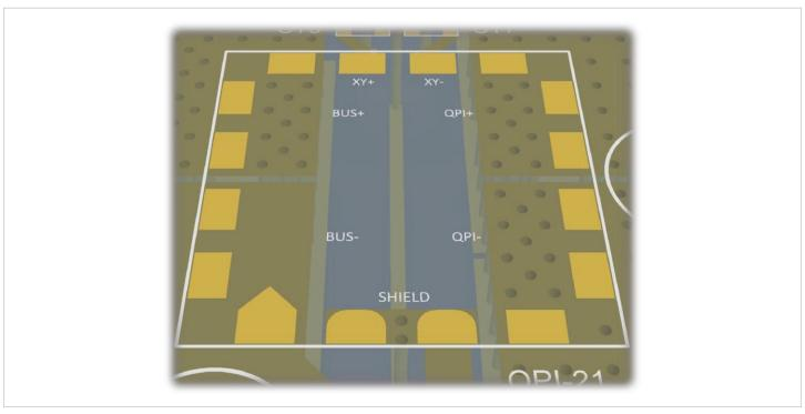
Figure 24 — 3D view of paralleling planes underneath the QPI-21
