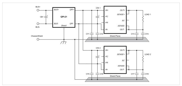
Figure 15 — The QPI-21 filtering dual supplies.[e]
