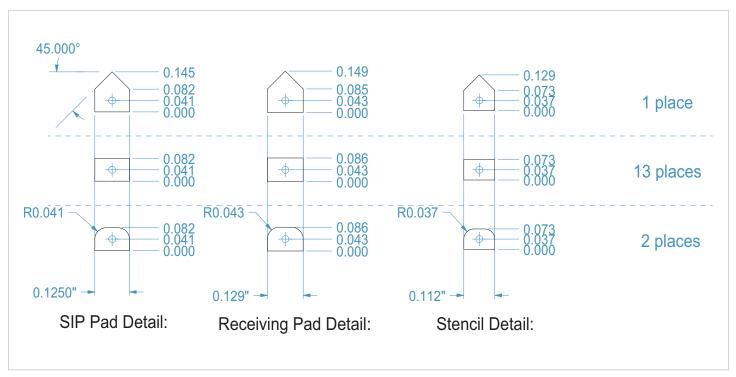
**Figure 23** — Recommended receptor and stencil patterns. (All dimensions are in inches.)
