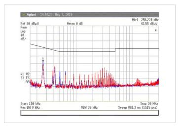
**Figure 7** — Ericsson PKM 4402NG using open-frame "Y" capacitors on QPI-21-CB1 evaluation board, 414 W load, converter's output ground connected to earth
