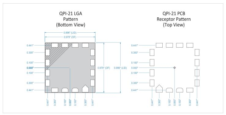
Figure 22 — Bottom view of open-frame (OF) and lidded (LID) products. (All dimensions are in inches.)
