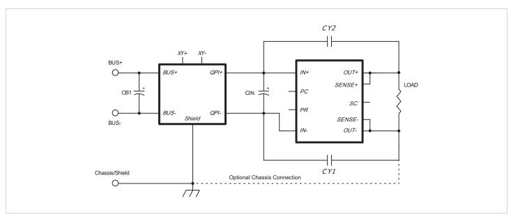
**Figure 5** — Typical "open-frame" application with an optional connection of the chassis to OUT- of the converter
