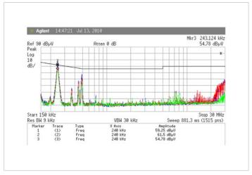
**Figure 10** — CM Peak Measurements with a 10  $\mu$ F and 47  $\mu$ F CX1 capacitor
