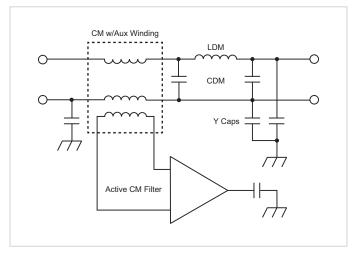
Figure 3 — Simplified Active EMI filter circuit
