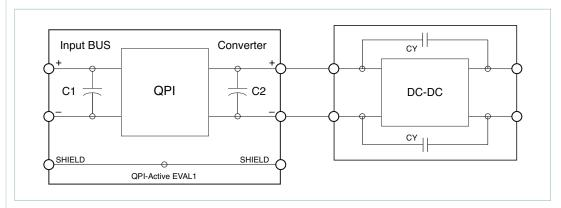
**Figure 2** Typical for "baseplate" EMI topology
