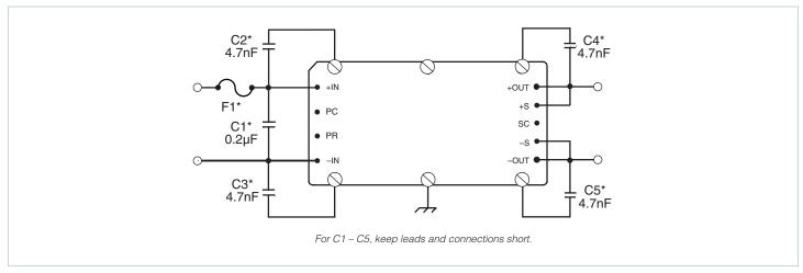
Figure 1 — Basic module operation requires fusing, grounding, bypassing capacitors.\* See Maxi, Mini, Micro Design Guide.
