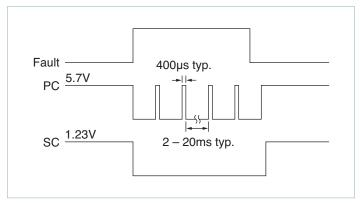
Figure 5 — PC/SC module alarm timing
