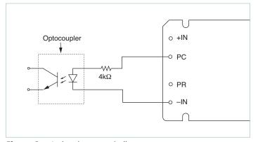
Figure 6 — Isolated on-state indicator
