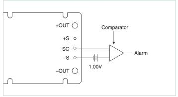
Figure 7 — Secondary-side on-state indicator
