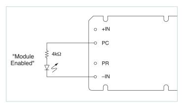
Figure 4 — LED on-state indicator
