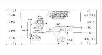
Figure 3 — PC/SC module alarm logic
