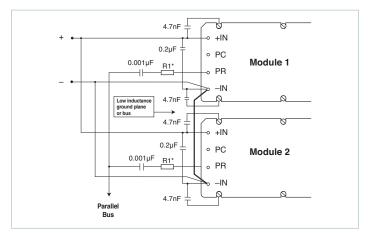
Figure 9 — AC-coupled single-wire interface
