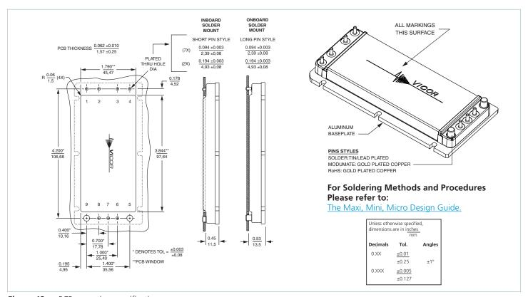
Figure 13 — PCB mounting specifications
