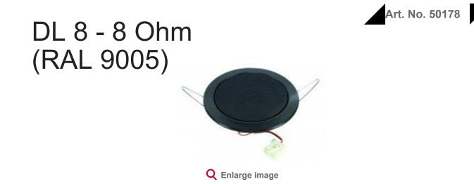
**8 cm (3.3") ceiling-mounted speaker** with black metal cover (RAL 9005). Suitable for use in all types of hollow ceilings. Easy fitting in round cut-out using spring arms, electrical connection by spring-loaded terminal clips. A compact solution for home and professional use with good sound qualities.
