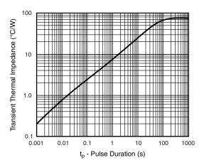
Fig. 5 - Typical Transient Thermal Impedance
