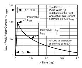
Fig. 3 - Pulse Waveform
