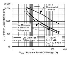
Fig. 4 - Typical Junction Capacitance Uni-Directional
