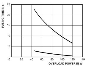
FUSING CHARACTERISTICS OF AC03-CS: 4.7  $\Omega \le R \le 100~\Omega$
