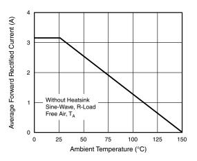
Fig. 2 - Forward Current Derating Curve
