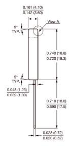
Polarity shown on front side of case, positive lead beveled corner
