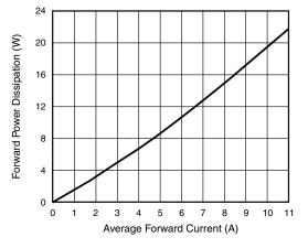
Fig. 3 - Forward Power Dissipation
