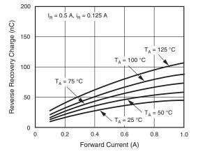
Fig. 7 - Reverse Recovery Charge vs. Forward Current
