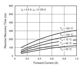
Fig. 6 - Reverse Recovery Time vs. Forward Current
