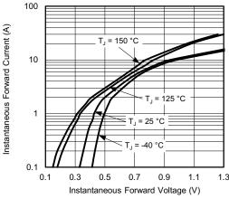
Fig. 5 - Typical Instantaneous Forward Characteristics
