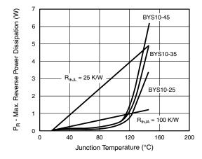
Fig. 1 - Max. Reverse Power Dissipation vs. Junction Temperature
