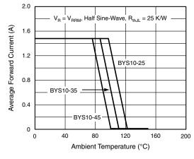
Fig. 3 - Max. Average Forward Current vs. Ambient Temperature
