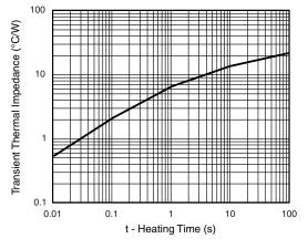
Fig. 6 - Typical Transient Thermal Impedance
