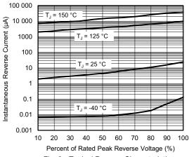
Fig. 2 - Typical Reverse Characteristics
