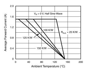
Fig. 4 - Max. Average Forward Current vs. Ambient Temperature
