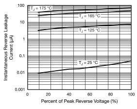
Fig. 5 - Typical Reverse Leakage Characteristics
