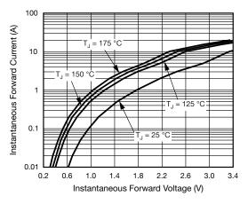
Fig. 4 - Typical Instantaneous Forward Voltage Characteristics
