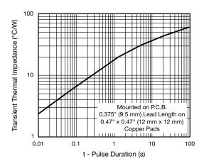
Fig. 7 - Typical Transient Thermal Impedance
