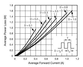
Fig. 2 - Forward Power Loss Characteristics
