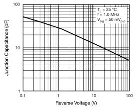
Fig. 6 - Typical Junction Capacitance
