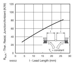
Fig. 1 - Max. Thermal Resistance vs. Lead Length
