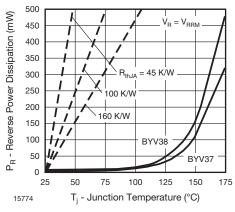
Fig. 2 - Max. Reverse Power Dissipation vs. Junction Temperature
