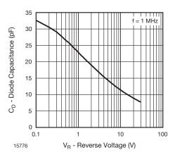
Fig. 6 - Typ. Diode Capacitance vs. Reverse Voltage
