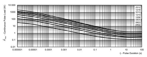
Maximum pulse load, continuous pulses; applicable if  $\bar{P} \leq P(\vartheta_{amb})$  and  $\hat{U} \leq \hat{U}_{max}$ ; for permissible resistance change equivalent to 8000 h operation
