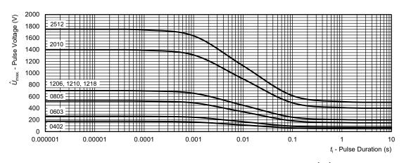
Maximum pulse voltage, single and continuous pulses; applicable if  $\hat{P} \le \hat{P}_{max.}$ ; for permissible resistance change equivalent to 8000 h operation
