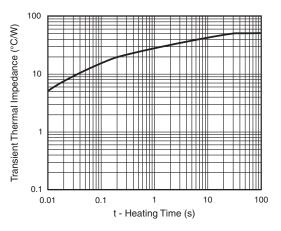
Fig. 6 - Typical Transient Thermal Impedance
