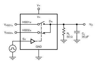
C<sub>L</sub> (includes fixture and stray capacitance)
