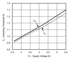
Switching Threshold vs. Supply Voltage
