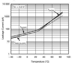
Leakage Current vs. Temperature
