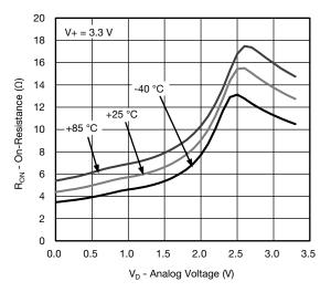
R<sub>ON</sub> vs. Analog Voltage and Temperature
