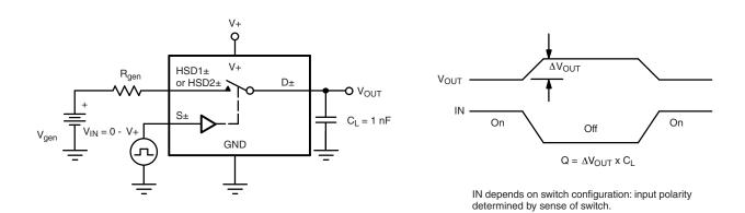
Fig. 3 - Charge Injection
