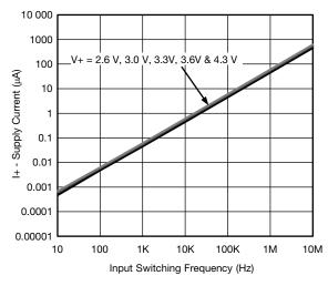
Supply Current vs. Input Switching Frequency
