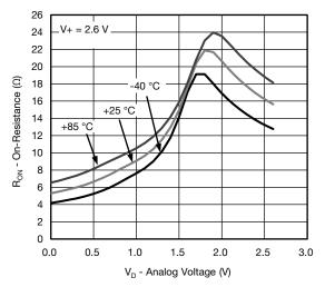
R<sub>ON</sub> vs. Analog Voltage and Temperature
