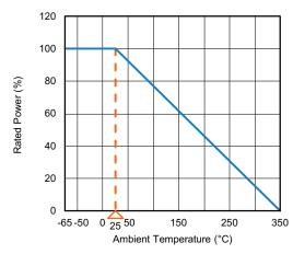
Derating is required for ambient temperatures above 25 °C per the above graph.
