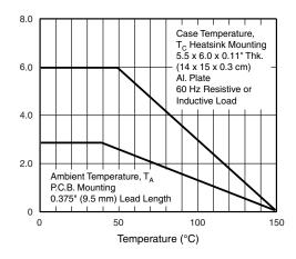
Fig. 1 - Derating Curve Output Rectified Current
