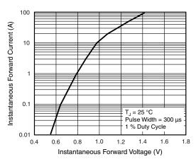
Fig. 3 - Typical Forward Characteristics Per Diode
