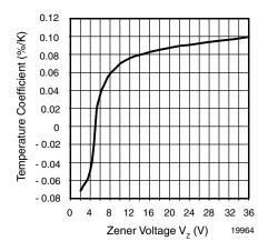
Fig. 1 - Zener Voltage Temperature Coefficient vs. Zener Voltage
