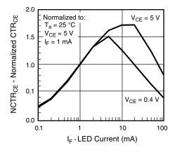
Fig. 13 - Normalized Non-Saturated and Saturated CTR<sub>CE</sub> vs. LED Current
