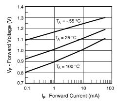
Fig. 1 - Forward Voltage vs. Forward Current
