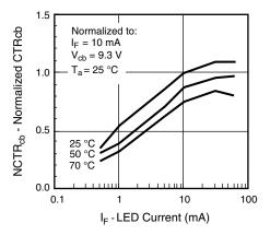
Fig. 8 - Normalized CTR<sub>cb</sub> vs. LED Current and Temperature
