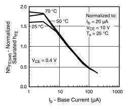
Fig. 11 - Normalized Saturated  $h_{\text{FE}}$  vs. Base Current and Temperature
