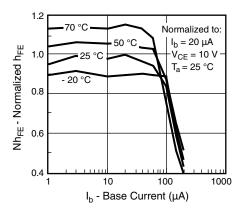
Fig. 14 - Normalized Non-Saturated  $h_{\text{FE}}$  vs. Base Current and Temperature
