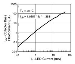
Fig. 9 - Collector Base Photocurrent vs. LED Current
