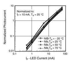
Fig. 10 - Normalized Photocurrent vs.  $I_F$  and Temperature
