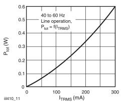
Fig. 9 - Power Dissipation 40 Hz to 60 Hz Line Operation
