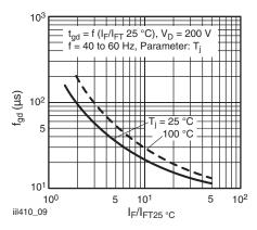
Fig. 7 - Typical Trigger Delay Time
