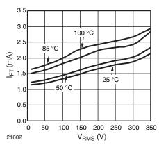
Fig. 11 - Trigger Current vs.
