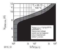
Fig. 10 - Typical Static Inhibit Voltage Limit
