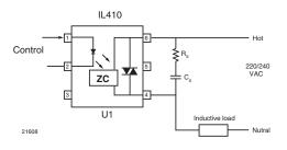
Fig. 15 - Basic Direct Load Driving Circuit
