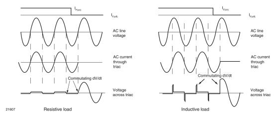
Fig. 12 - Waveforms of Resistive and Inductive Loads
