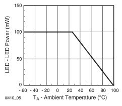
Fig. 3 - Maximum LED Power Dissipation
