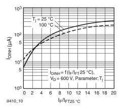
Fig. 8 - Off-State Current in Inhibited State vs.  $I_F/I_{FT}$  25 °C
