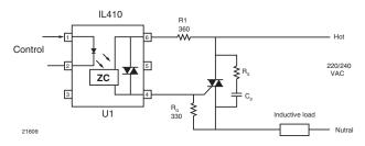
Fig. 16 - Basic Power Triac Driver Circuit
