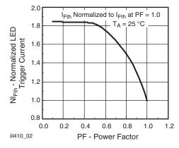
Fig. 14 - Normalized LED Trigger Current vs. Power Factor
