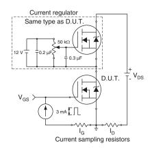
Fig. 13b - Gate Charge Test Circuit
