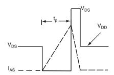
Fig. 12b - Unclamped Inductive Waveforms
