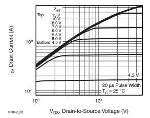
Fig. 1 - Typical Output Characteristics, T<sub>C</sub> = 25 °C
