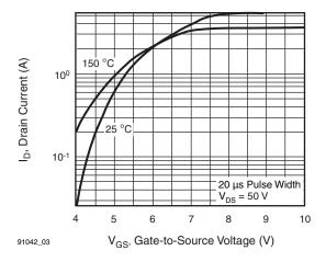
Fig. 3 - Typical Transfer Characteristics
