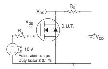
Fig. 10a - Switching Time Test Circuit
