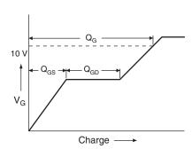
Fig. 13a - Basic Gate Charge Waveform
