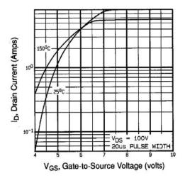
Fig. 3 - Typical Transfer Characteristics
