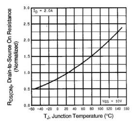
Fig. 4 - Normalized On-Resistance vs. Temperature
