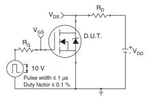
Fig. 10a - Switching Time Test Circuit
