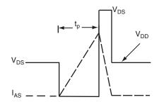
Fig. 12b - Unclamped Inductive Waveforms
