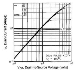
Fig. 2 - Typical Output Characteristics,  $T_C = 150$  °C
