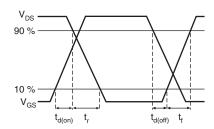
Fig. 10b - Switching Time Waveforms
