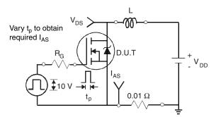
Fig. 12a - Unclamped Inductive Test Circuit
