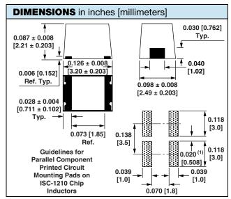
Recommended minimum spacing between components
