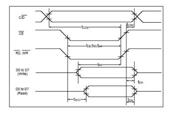
(VDD=+5V $\pm$ 5%,GND=0V,Ta= -20 to +70°C)
